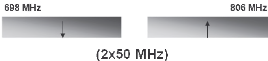
Fig. 5. 2 \times 50 MHz FDD arrangement for 700 MHz band plan
