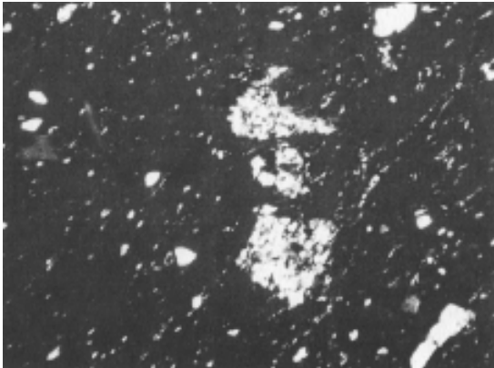
Fig. 2. Sample MD 2112. The matrix is isotropic, strongly changed thermally; clastic material: quartz, some pores with rims from cryptocrystalline carbonates, rock fragments. The sample was originally fired at 1000-1050°C. Microphotos, XPL. Bar represents 200μm.
