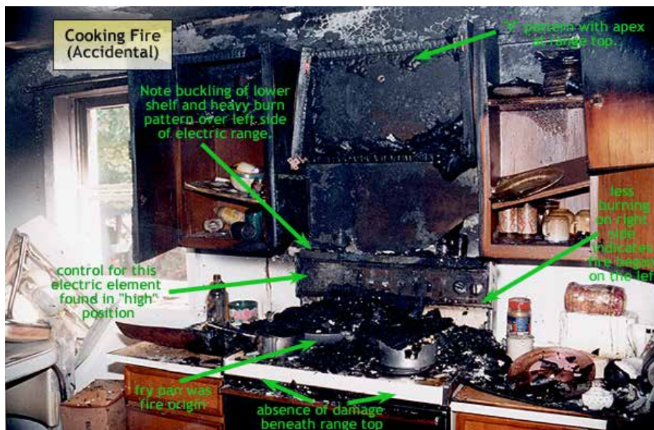
FIG. 4. TRAINING FIRE INVESTIGATION SITE WITH THE KITCHEN
