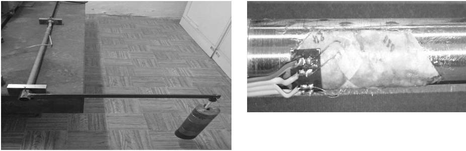
Fig. 3. Rod loaded by torsion and location of strain gauges
