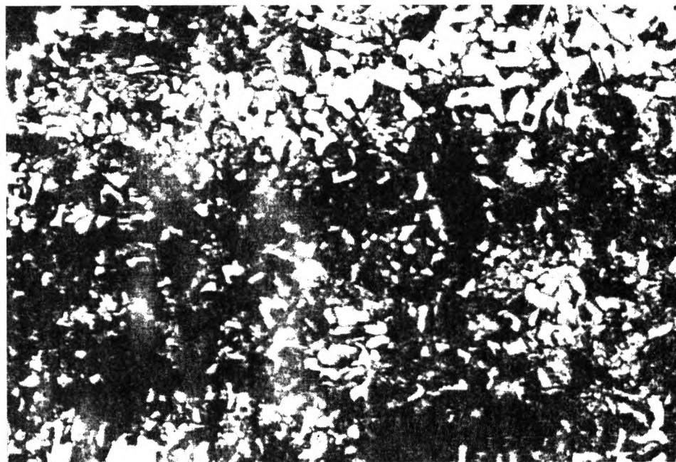
Fig. 6. Structure of steel edge of knife No 6. Nital etched, 500x.
