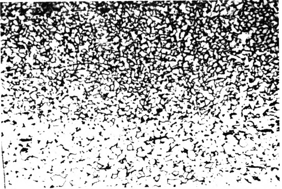
Fig. 9. Structure of knife No 7 made of fine grained iron, Nital etched, 500x.
