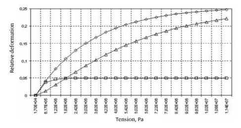
Drawing of dependence of relative deformation of soil on tension in the range from 0,02 MPa to 12,02 MPas for various approximating functions.
