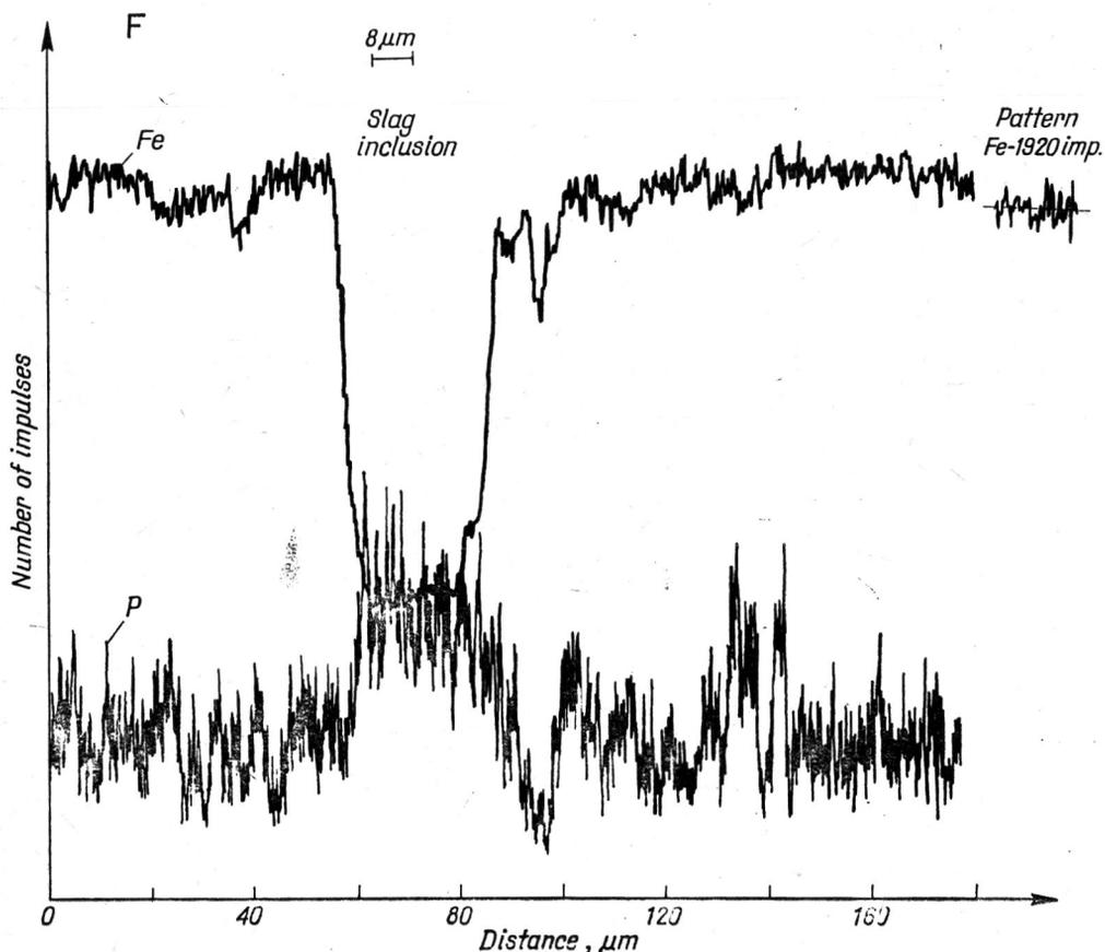
Fig. F. Diagram of changes in the content of Fe and P in the Malayan creese
