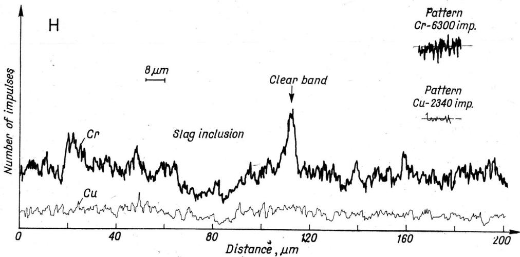
Fig. H. Diagram of changes in the content of Cu and Cr in the Malayan creese
