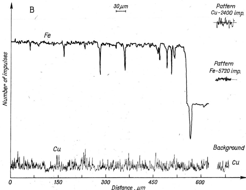
Fig. B. Diagram of changes in the content of Fe and Cu in knife no. 5 from Czeladź Wielka, Góra district (9th - 12th cent.)
