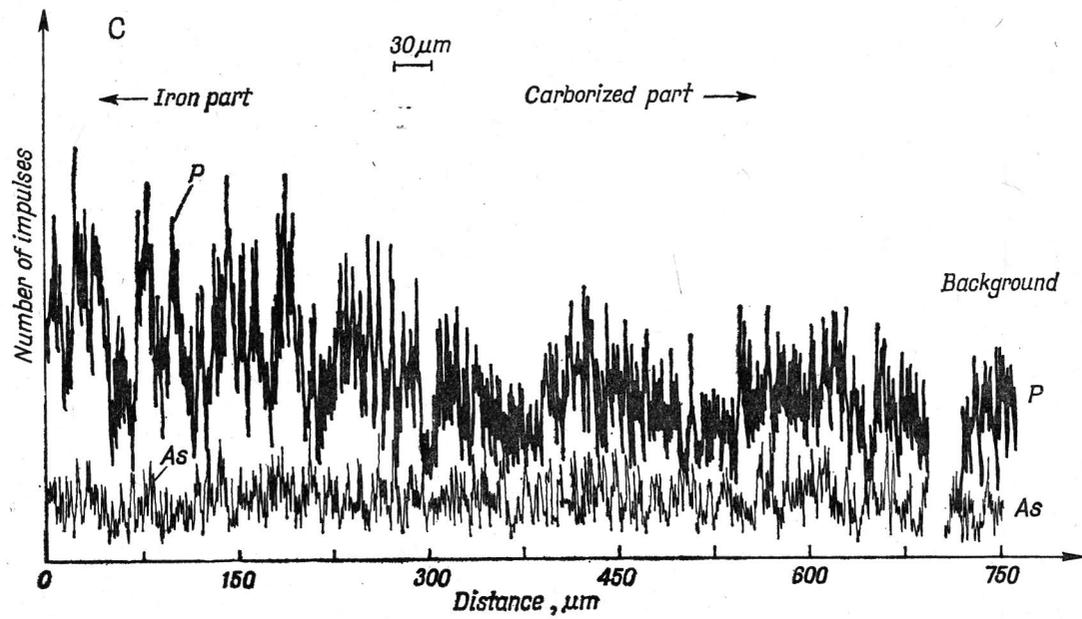
Fig. C. Diagram of changes in the content of P and As in knife no. 5 from Czeladź Wielka, Góra district<sup>t</sup> (9th - 12th cent.)
