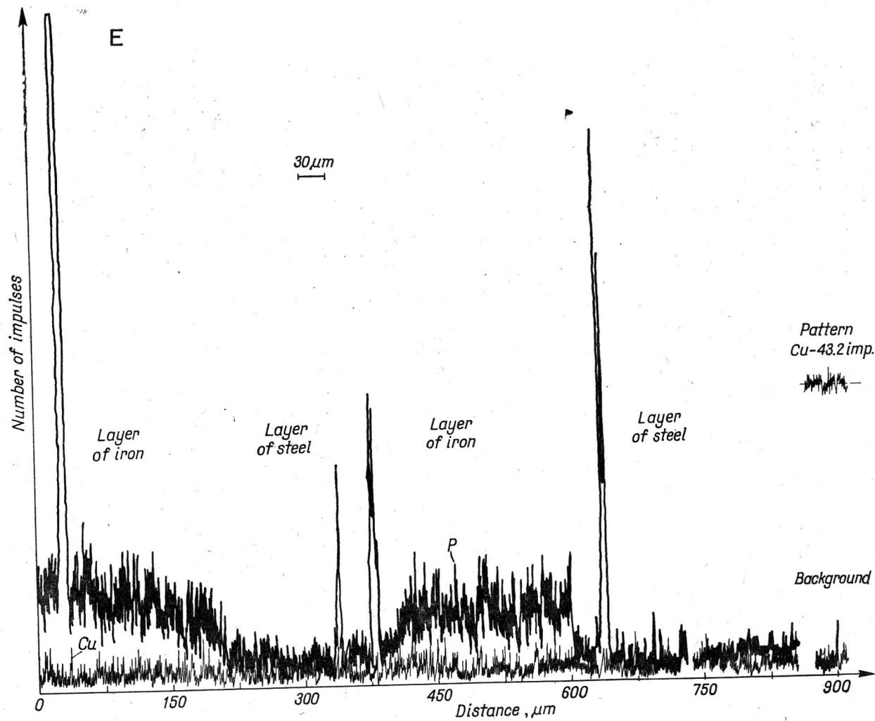
Fig. E. Diagram of changes in the content of P and Cu in the Roman sword from Sobótka, Łęczycza district (2nd - 3rd cent.)
