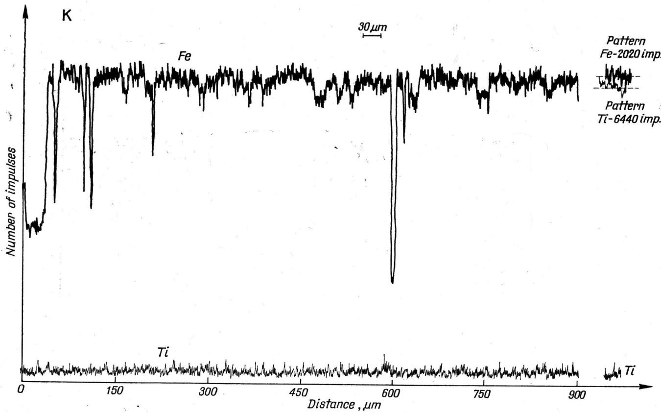
Fig. K. Diagram of changes in the content of Fe and Ti in the socketed axe from Jezierzycy, Dzierżoniów district
