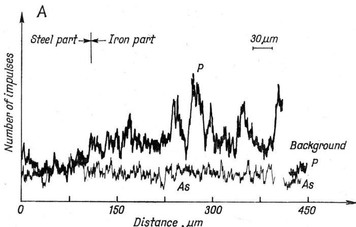
Fig. A. Diagram of changes in the content of P and As in knife no. 3 from Piekary, Cracow district (13th cent.)
