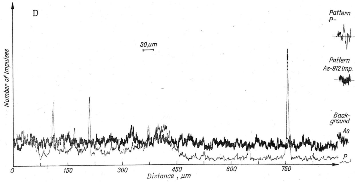
Fig. D. Diagram of changes in the content of P and As in the axe from Nowa Huta-Mogila (Roman period)
