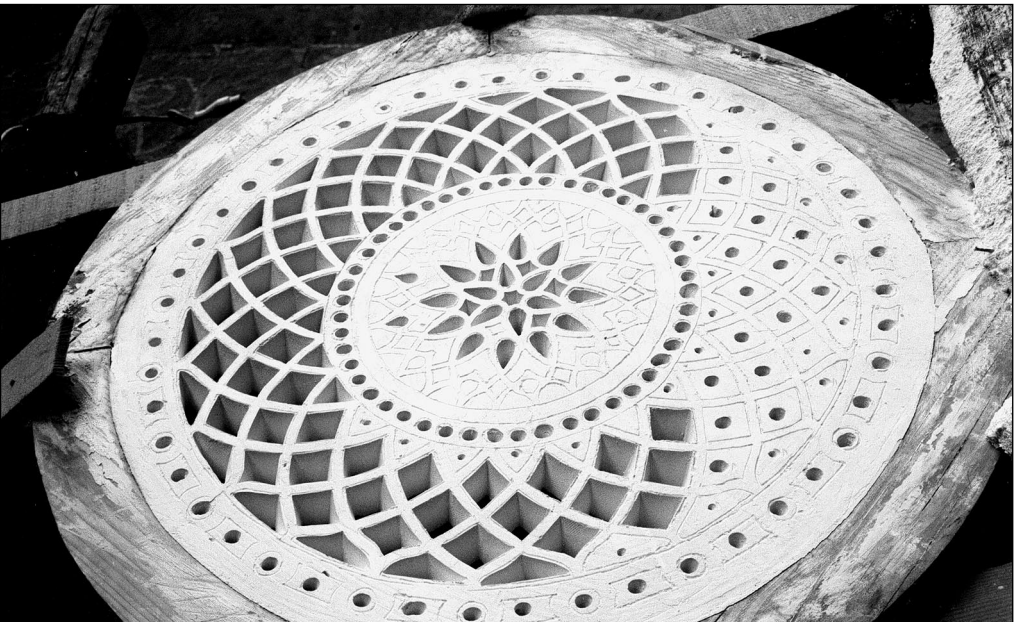
Fig. 6. Qubba. Qammariyyat workshop. Detailed view of a round qammariyya being prepared for the oculus in the mausoleum dome (Photo J.J. Kania)
