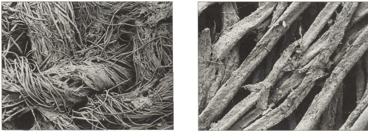
Fig. 1. Series I. Undyed fabric (3) woven with handspun wool before and following 11 years' burial in a lidded oak box in the bog at Lejre. left – fabric following burial; right – fibres following burial exhibiting extensive biodeterioration. Scanning electron photomicrograph E. Peacock.
