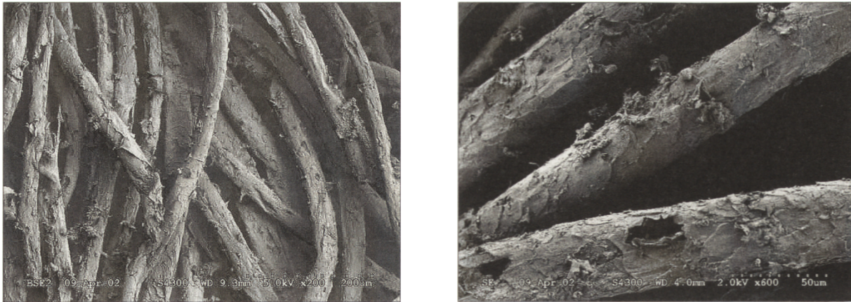
Fig. 5. Wool fabric (madder-dyed) following two years' unprotected burial in the bog at Lejre. The fibres illustrate morphological changes characteristic of biodeterioration. Scanning electron photomicrograph E. Peacock.
