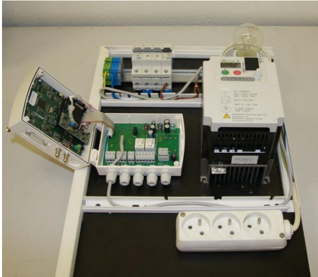
Fig. 4. Model of regulation of illumination of the remote experiment in the real laboratory
