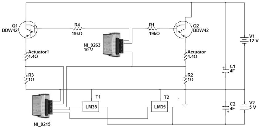
Fig. 8. Control circuit of SMA actuators
