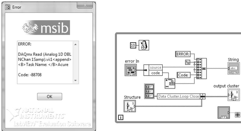
Fig. 12. Error message and its source code (one of the 22 subprograms)
