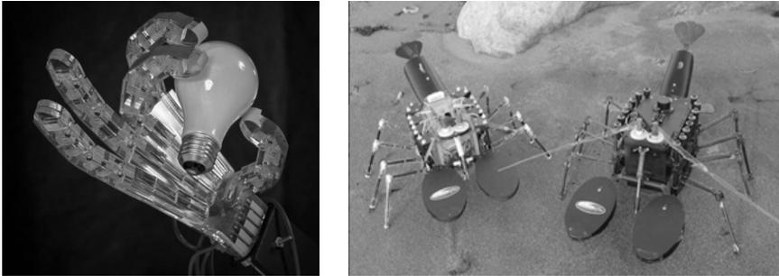
Fig. 1. Artificial hand and mobile robots driven by SMA wires
