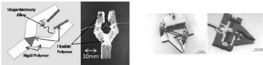
Fig. 2. Mini grippers driven by SMA springs
