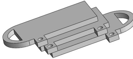
Fig. 5. The internal construction of the SMA actuator with linear activation of SMA wires
