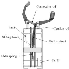
FIG. 1. Mechanical structure of the gripper.
