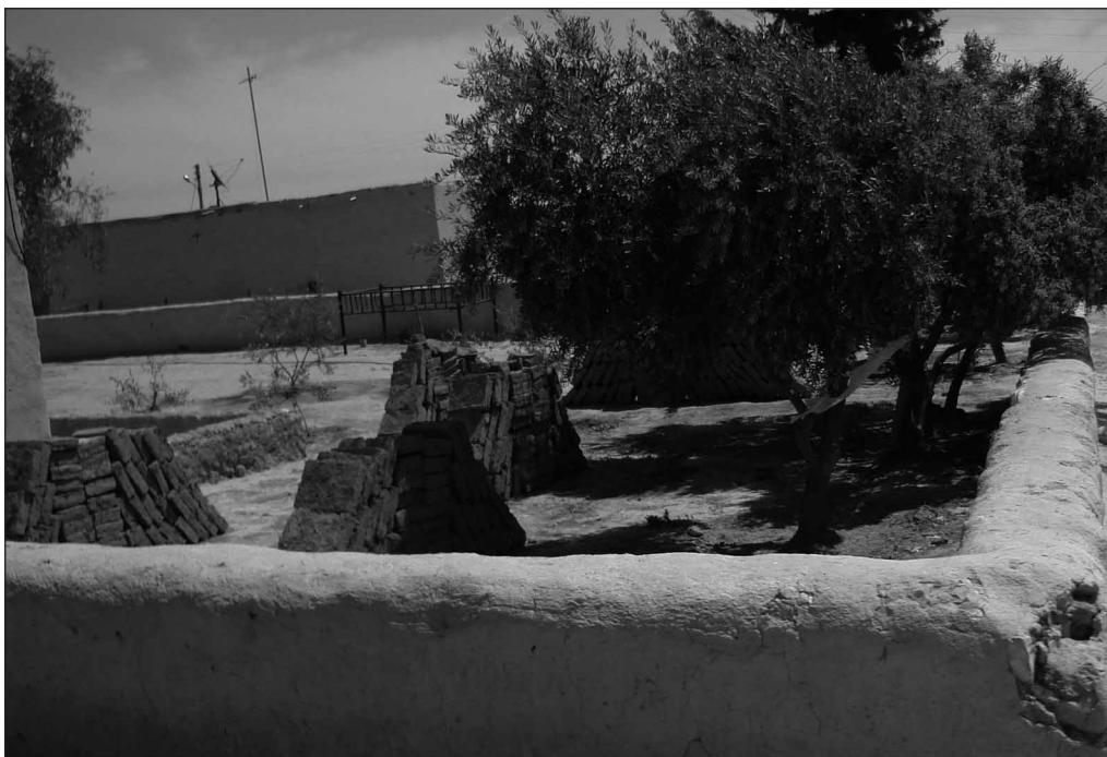
Fig. 5. Modern sun-dried mud bricks in a Syrian village on the Middle Euphrates (Photo M. Białowarczuk)
