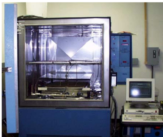
Fig. 11. The test apparatus - hotplate in an environmental chamber [1]
