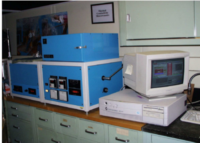
Fig. 5. Apparatus for testing the thermal conductivity - Rapid-k together with the computer system [9, 10]
