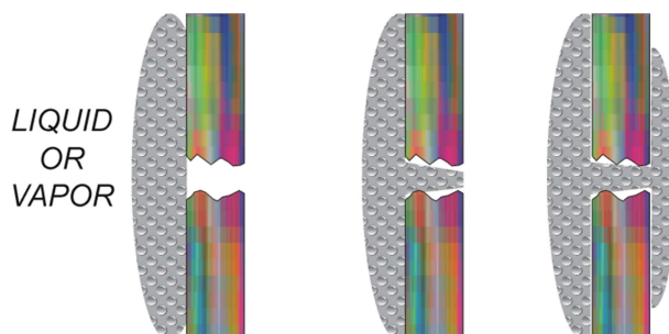
Fig. 13. Illustration of penetration chemical or liquids vapors through the material [1]
