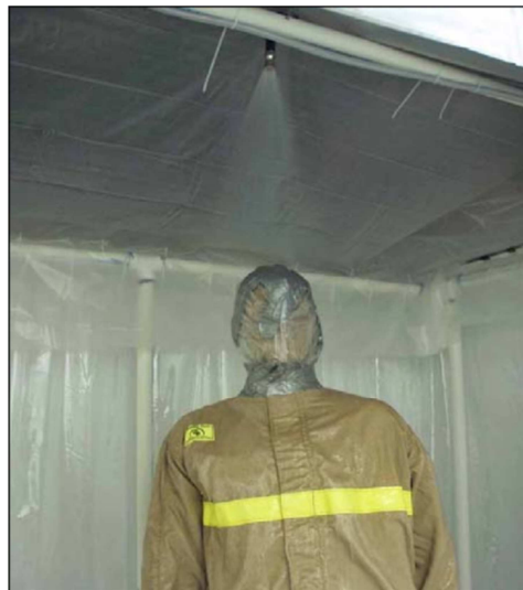
Fig. 15. Test of penetration the fire protective clothing by liquids [1]
