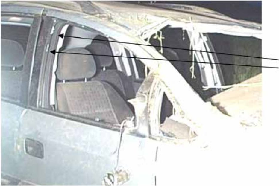
The glass remains trapped in the guide seal of the RF door
