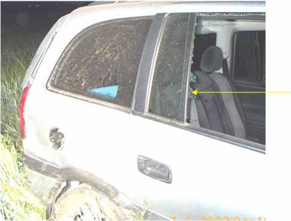
The glass remains trapped in the guide seal of the RR door
