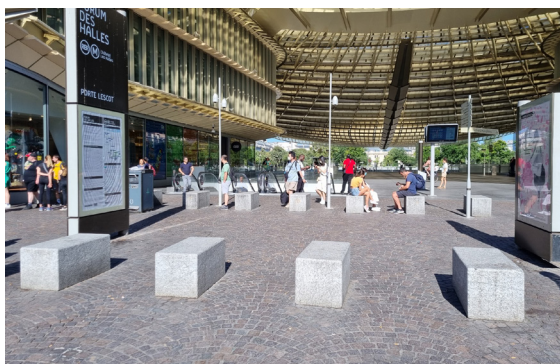
Image 7. Concrete barriers – a solution with organisational or potentially protective function. Whether they are classified as VSBs depends on their certification and the scenario in which they are used (Paris).
